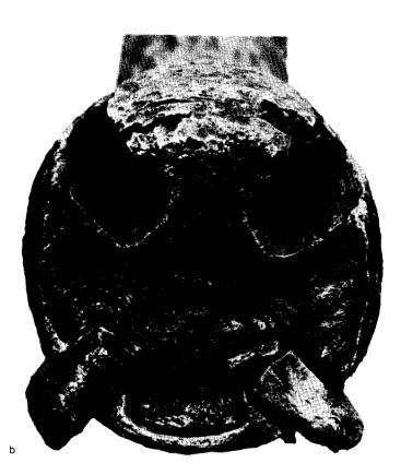
$Fig. 66 \quad Boring\ bar\ from\ Stream\ furnace, Chiddingly\ (TQ\ 555155).\ This\ wrought-iron\ bar\ (a)\ probably\ dates\ from\ the\ seventeenth\ century.\ Its\ head\ (b)\ had\ originally$ contained four cutters, three of which were in position when the bar was recovered (see Butler and Tebbutt 1975) (scale on bar: 1ft) (photograph: D. S. Butler).
